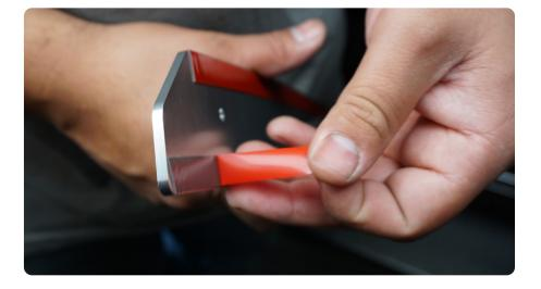
**STEP 2** | Install the sill by pressing it firmly into place.
