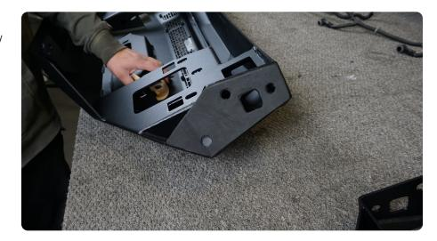
STEP 16 | Use the provided M12x30 hardware to secure the wings to the bumper, ensuring they are aligned properly.
