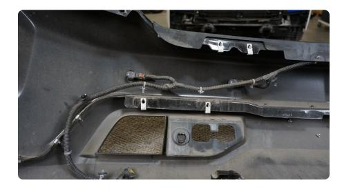
STEP 13 | Remove the sensors from the bezels by gently spreading the locking tabs to release the sensor from the bezel.
