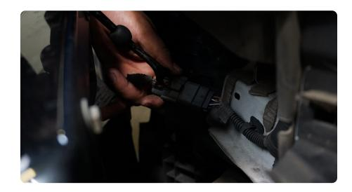
STEP 6 Use a 10mm socket with a 10" extension and swivel socket to remove the various hardware securing the bumper to the vehicle.
