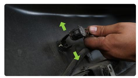
STEP 14 Use a pick or similar to carefully press the retaining tabs around the sensor bezel to gently push it out of the front of the bumper.
