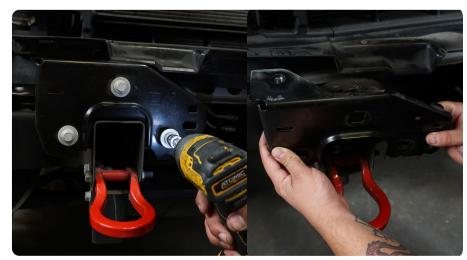
STEP 9 | Use an 18mm socket/wrench to remove the hardware securing the tow hook and set it off to the side.
