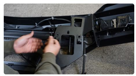
STEP 19 | Install the sensor bezels in the locations and orientation they were removed from the factory bumper.
