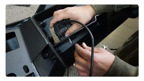
STEP 18 | Install the provided M12 nut clips by pressing them into place.
