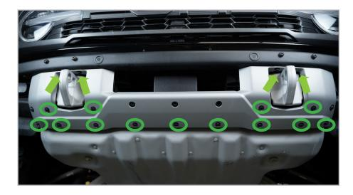
Pull the D-ring guard away from the Bronco firmly and set to the side.
