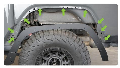
STEP 15 | Install the Rear Fender Delete onto the vehicle using the provided M6x25 hardware with a 4mm allen bit (and 10mm wrench if using nuts).
