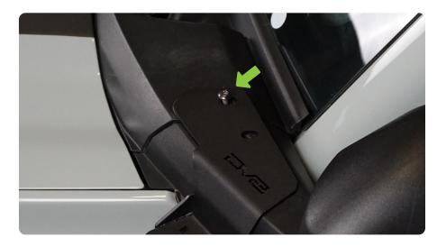
STEP 4 | Passenger side: Guide antenna through the DV8 mount and lay the mount into place, then loosely secure the DV8 mount to side mirror.
