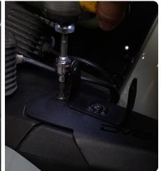
STEP 6 Optional: A set of additional mounting tabs are included in the kit, these tabs allow Antennas, Whips and etc... to be installed.
