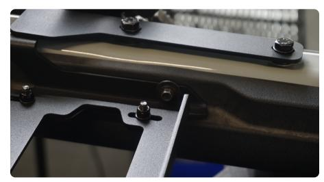
STEP 19 | Use a 13mm socket or T50 Torx bit to secure the hardware holding the mounting plate to the roll-bar.
