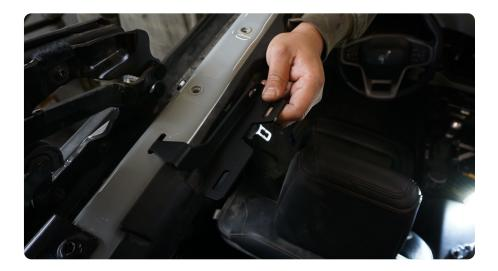
Loosely install the pressure plate.
