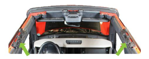
STEP 13 | Use a 8mm wrench to remove the bolt on the interior of the roll bar.
