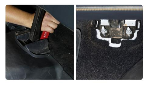
STEP 5 | Use a 13mm socket to remove the two bolts.
