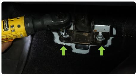
STEP 6 | Place mounting bracket over the studs and using factory bolts and a 13mm, loosely secure bracket.
