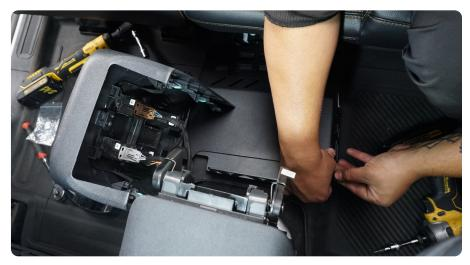
**STEP 8** Reinstall the center console at this time by aligning the tabs and pressing firmly until they "click" into place.
