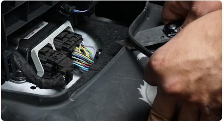
Mounting bracket should lay flat once completed.
