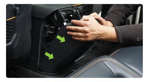
STEP 2 | Place the mounting bracket over the driveshaft tunnel. Use a marker to show where the mat will be trimmed.
