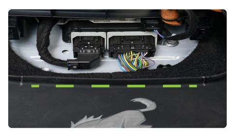
STEP 3 Using a razor blade or similar sharp tool to cut, trim along the lines marked in previous step.
