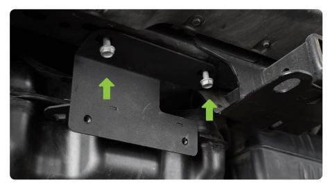
STEP 11 | Place the nut plate for the passenger side support bracket into the hitch and loosely secure the bracket using the provided M12 hardware with a 6mm allen bit.
