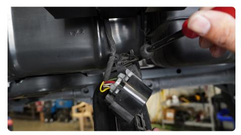
**STEP 3** Use a 13mm socket to remove the bolts securing the factory skid plate to the DEF tank and set it off to the side.
