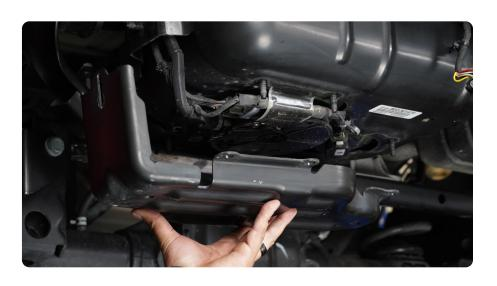
**STEP 4** | Place a support under the DEF tank/assembly to prepare for removal of the final support brace.
