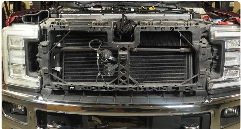
**STEP 4** | Using a trim clip tool to remove the ACC module cover.
