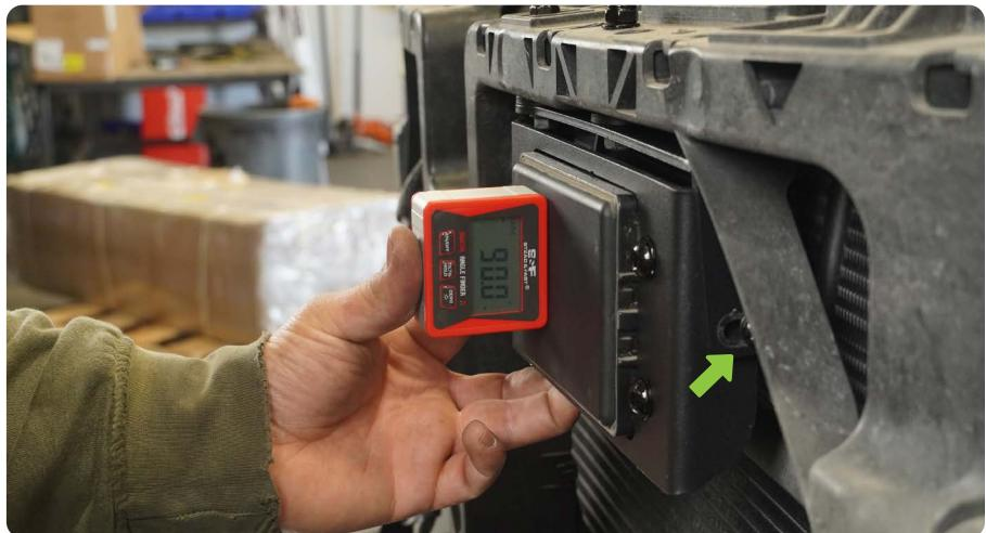
**STEP 15** | Install the grille back onto the vehicle. Use cutters to clearance the grille mounting bracket for the modules mounting bolts.
