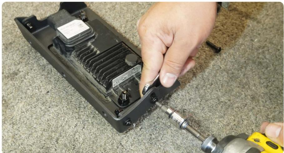
**STEP 13** | Using the provided M8x50mm hardware, mount the ACC module to the radiator support.
