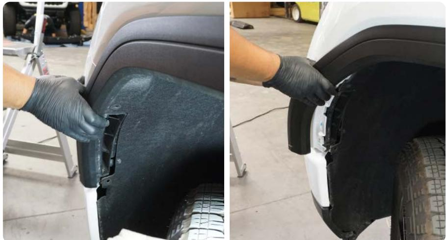
**STEP 6** | Using a 7mm socket, remove the bolt that secure the lower fascia to the fender on each side.
