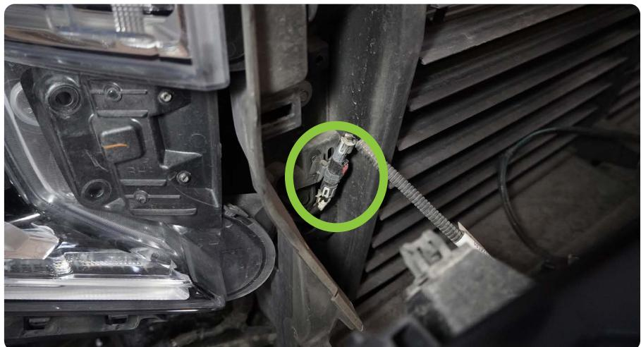
**STEP 10** | If your vehicle is equipped with an illuminated grille emblem, disconnect the (2) electrical plugs behind the driver side headlight.
