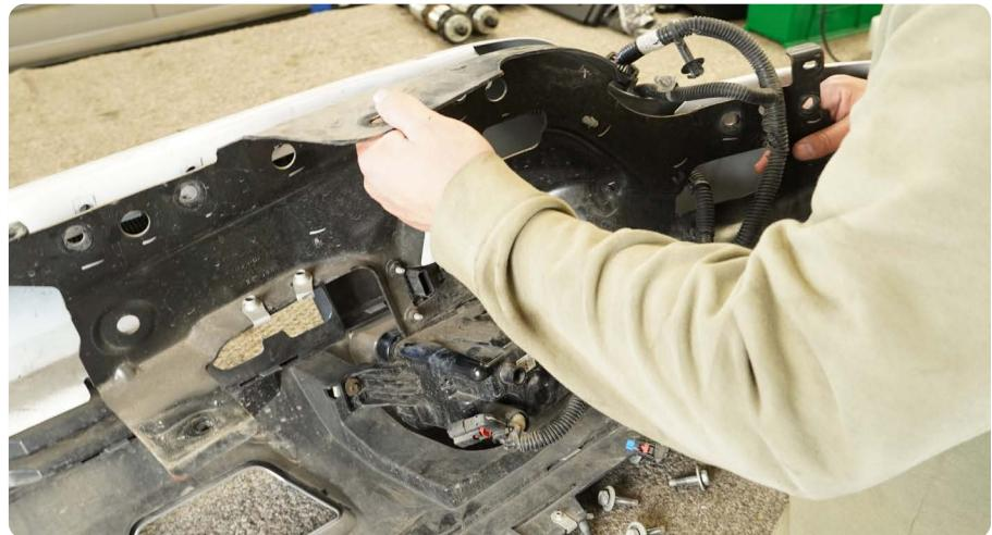
**STEP 20** | Using a 10mm socket, remove the bolts that secure the ACC module to the bumper support.
