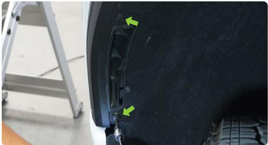
**STEP 5** | With a firm grip, carefully, pull the front of fender flare away from the vehicle body.
