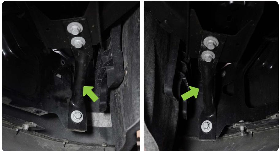
**STEP 14** | Use an 18mm socket to remove the (2) lower bumper mounting bolts on the inside of the frame rails.
