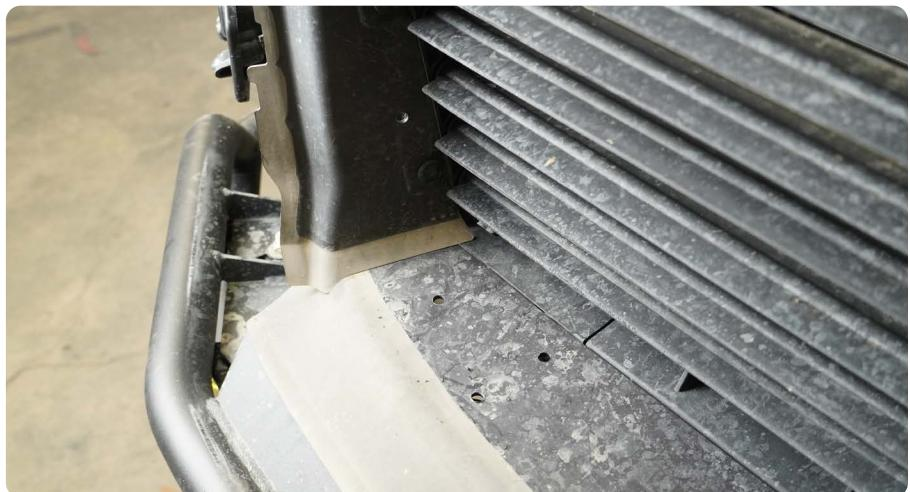
**STEP 29** | Mount the relocation bracket to the shutter system shroud using the rest of the M6 hardware.
