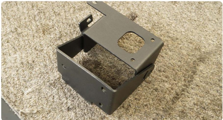
**STEP 22** | Using 3 of the provided M6x20 allen head bolts and the M6 hardware provided secure the two brackets together.
