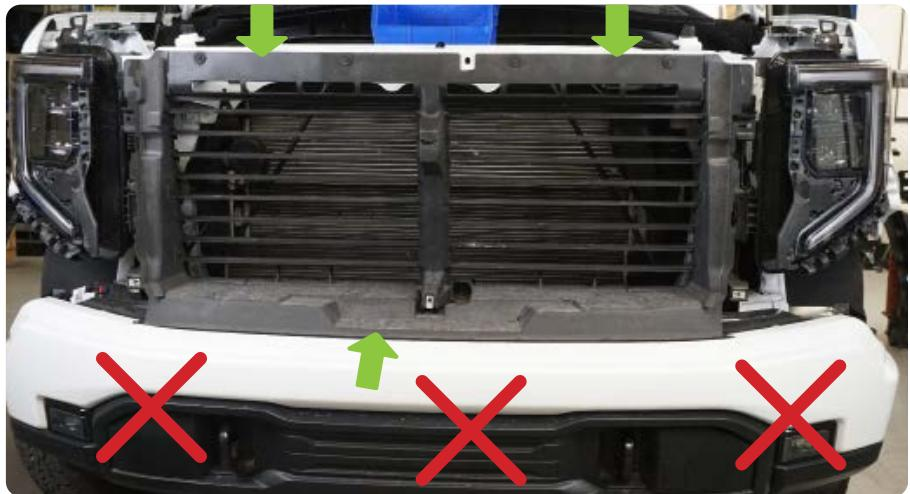
**STEP 26** | Place the ACC module and relocation bracket onto the passengerside front corner of the shutter system as shown.
