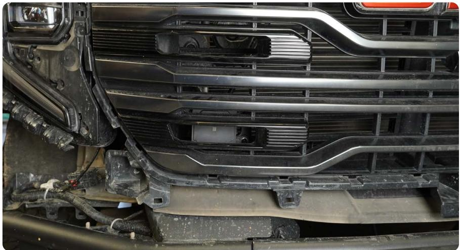
**STEP 33** | Congratulations, installation of the DV8 Super Cruise ACC module relocation bracket is now complete.
