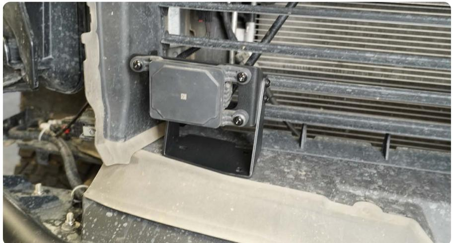
**STEP 27** | Use a marker to mark the 4 holes that will need to be drilled out.
