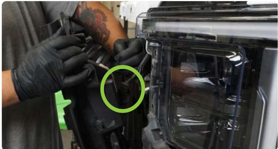
**STEP 12** | Disconnect the bumpers wiring harness located below the passenger headlight. Pull back the red locking tab and depress the push tab to separate the two electrical plugs.
