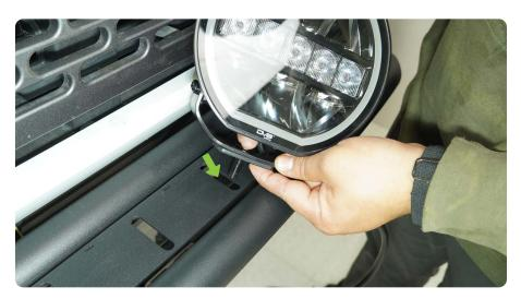
STEP 4 | Use the provided nylon lock nut to loosely secure the LED light in place.
