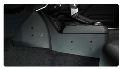
STEP 4 | Align the driver side mount with the holes secure molle using the provided M5 hardware.
