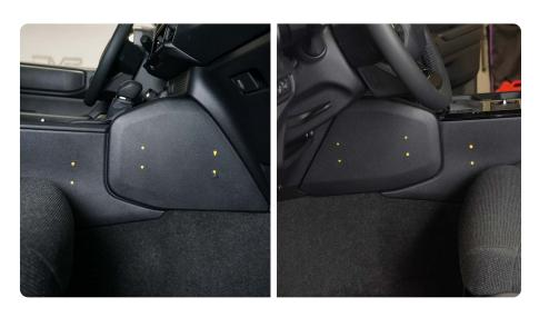
STEP 2 Use a 11/32" drill bit to drill out the (6) mounting holes on each side.
