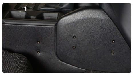
STEP 4 | Mount the DV8 Center Console Molle Panel on to the factory center console using the provided M6 Allen head bolts and flat washers.
