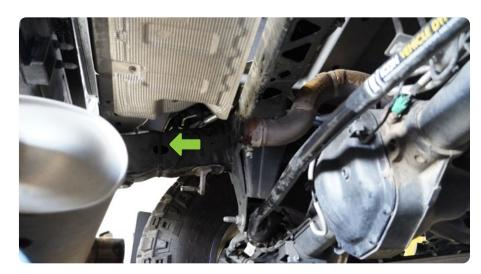
STEP 11 Use a 10mm socket and a trim clip tool to remove the factory hardware and plastic clip retainers securing the factory heat shield in place.
