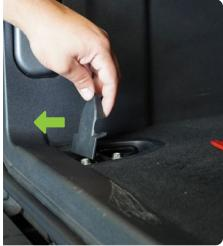
STEP 5 Use a 10mm socket to remove the hardware securing the factory tie-downs to the vehicle.
