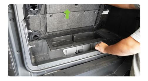
STEP 7 Use a 10mm socket to remove the hardware securing the factory storage box to the vehicle.
