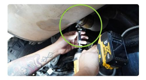
STEP 20 | Install the factory tiedowns using a 10mm socket and the factory hardware.
