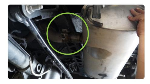
STEP 18 | Finish securing the muffler by re-installing it onto the hangers.
