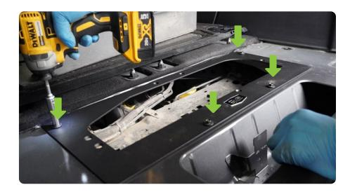
STEP 13 | Place the DV8 storage box under the vehicle and lift it to the mounting plate by reaching down through the empty space in the cab.
