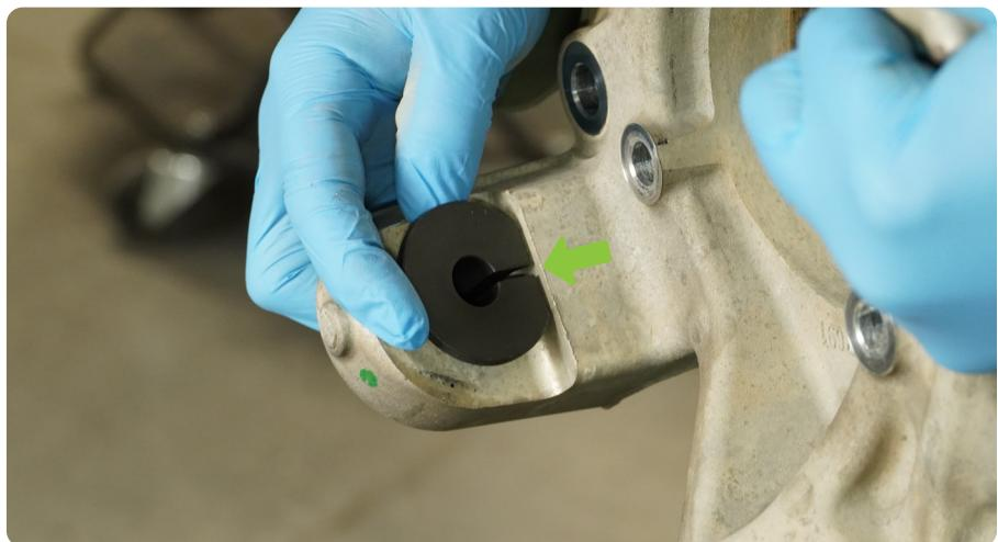
**STEP 26 |** Install the knuckle onto the DV8 ball joints. Loosely thread the lower ball joints castle nut onto the ball joint to hold the knuckle in place. Do not tighten the lower ball joint castle at this time.
