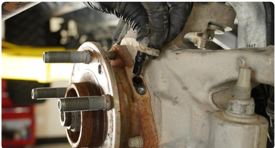
**STEP 8** | Using a 21mm socket remove the drag link and tie rod from the knuckle.
