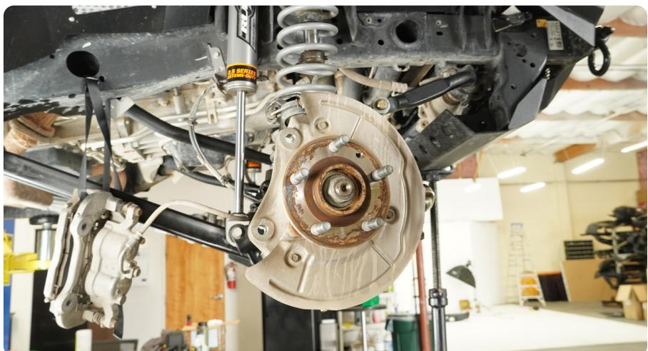
**STEP 5 |** Using a 10mm socket remove the brake dust shield.
