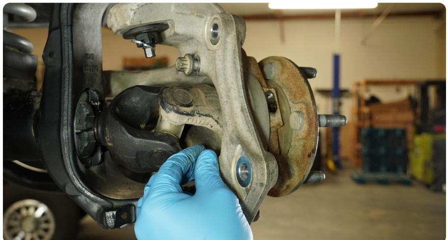
**STEP 31** | Using a torque wrench and an 12 point 13mm socket, torque the wheel hub bolts to 7 ft. lbs.
