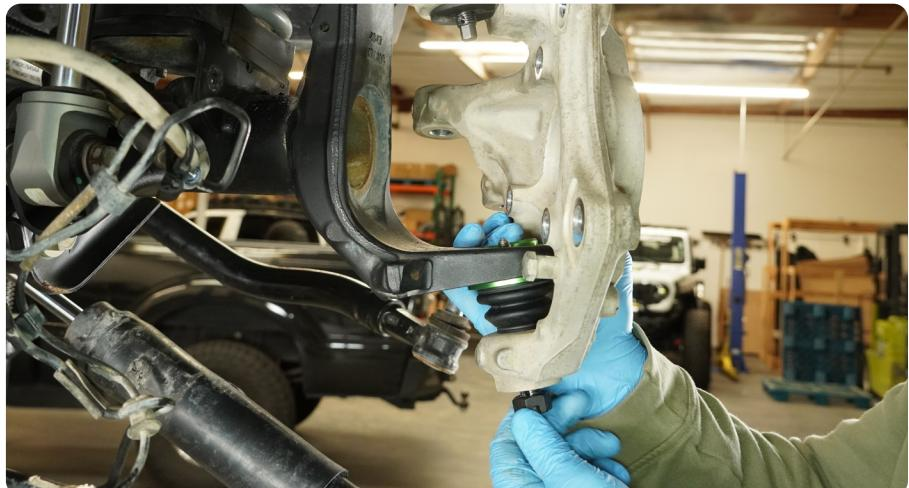
**STEP 27 |** Loosely thread the upper ball joints castle nut onto the ball joint.
