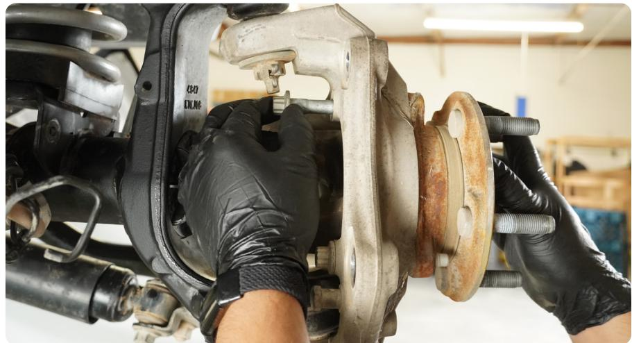
**STEP 14** | Remove the wheel hub and axle. If the wheel hub is stuck in place due to surface rust, use a hammer to tap the hub out of the knuckle.
