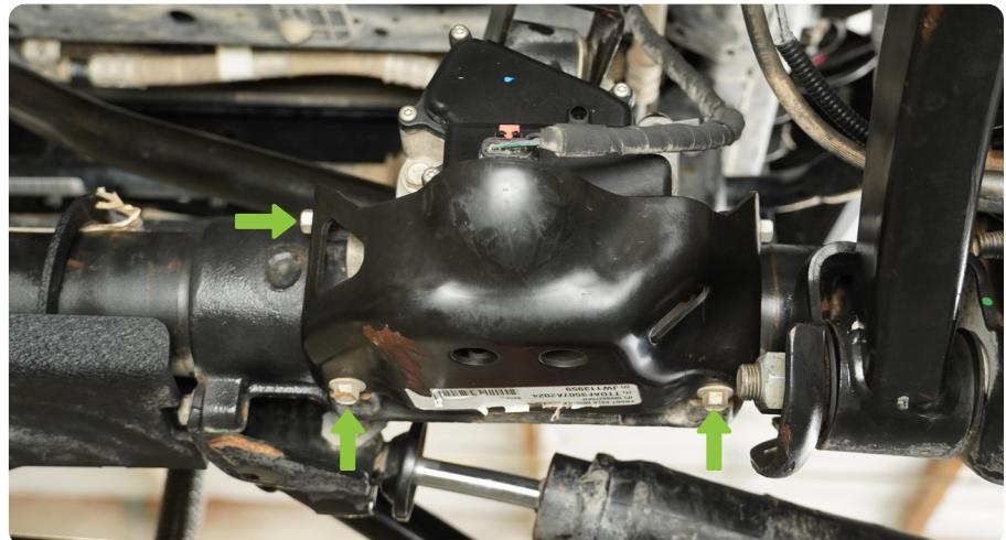
**STEP 10 |** Disconnect the motor wiring harness by pulling the red tab back and depressing the release tab.
