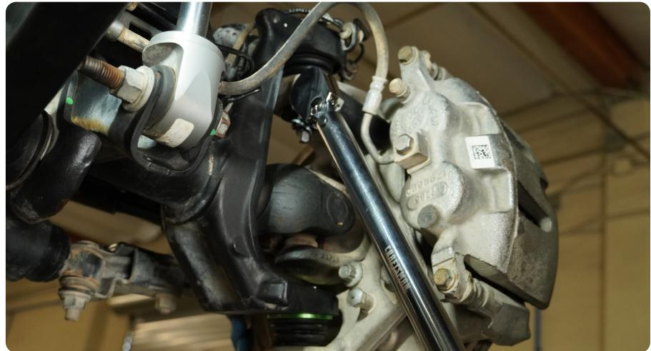
**STEP 37** | Secure the brake line bracket to the axle using the factory hardware and a 10mm wrench.
