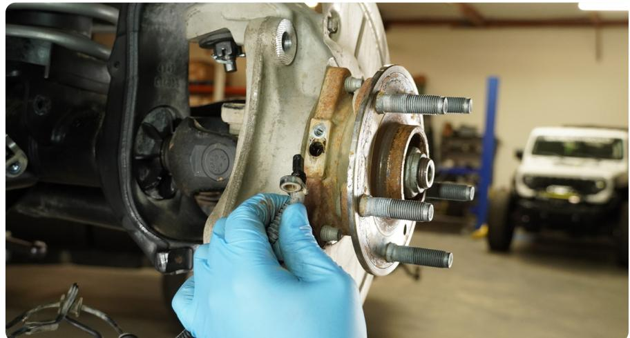
**STEP 36** | Re-install the brake rotor. Secure the rotor to the wheel hub using the factory set screw. Torque the set screw to 15 ft. lbs.
