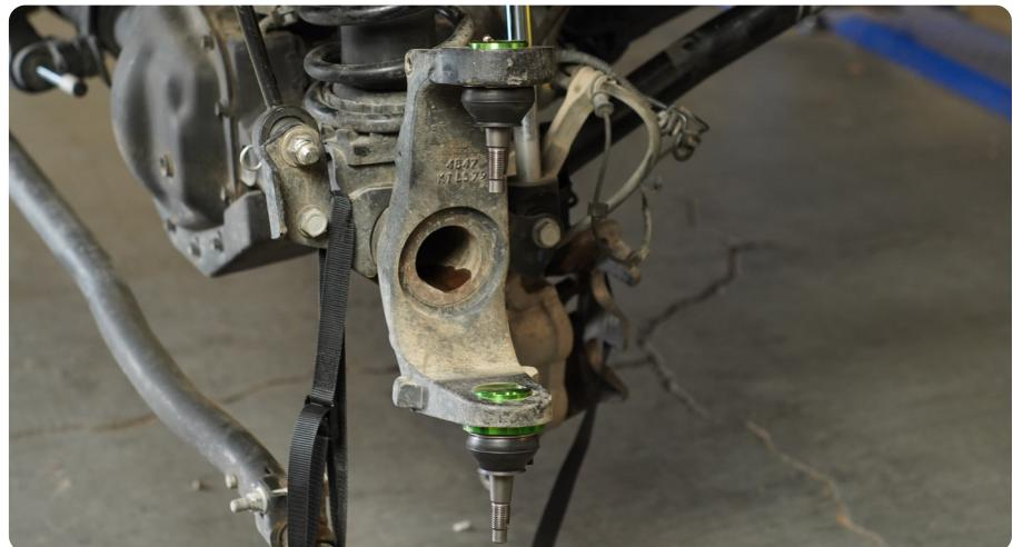
**STEP 40** | We provide flush and standard zerk fitting. Either style can be ran on either ball joint. For our install we used the flush on the lower and standard on the upper.
