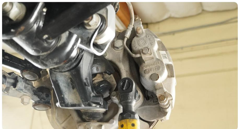
**STEP 3** | Using a T30 torx bit, remove the brake rotor screw.
