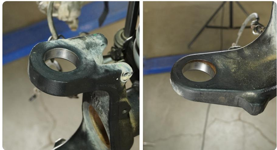
**STEP 21** | The DV8 ball joints are marked UPR (Upper) and LWR (Lower). Insert the lower ball joint into the axle first.
