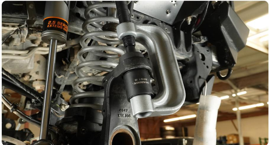
**STEP 24** | Ensure the ball joint is fully seated into place.
