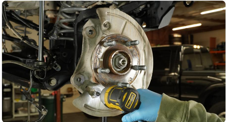
**STEP 35** | Using the factory hardware and a #5 allen tool, re-install the wheel speed sensor in to the wheel hub. Torque the speed sensor bolt to 5 ft. lbs.
