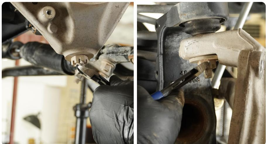
**STEP 16** | Using a 22mm socket remove the ball joint castle nuts.
