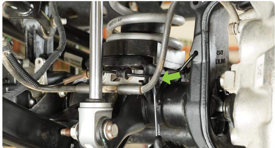
**STEP 38** | Secure the ABS line bracket using a 13mm socket.
