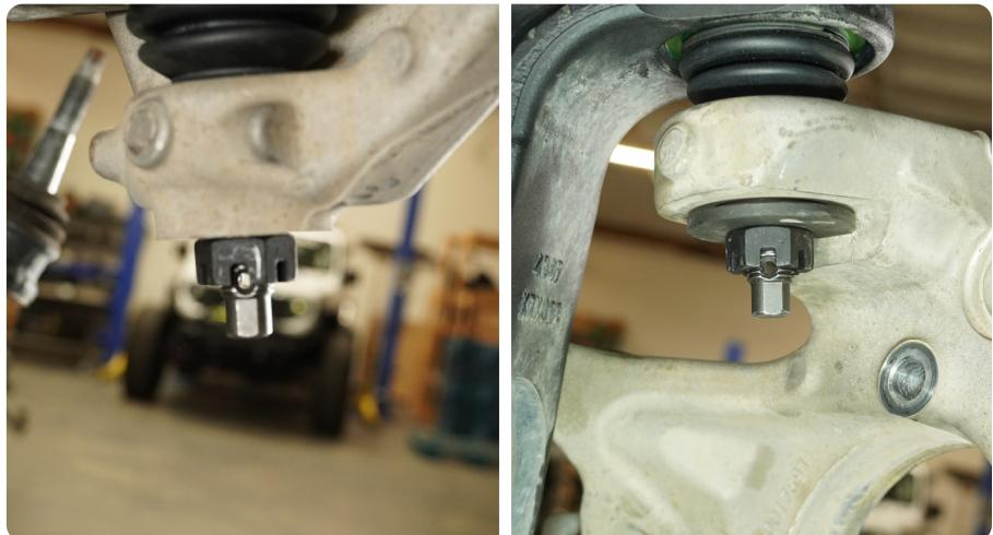
**STEP 29** | Install the provided cotter pins through the castle nuts to prevent the castle nuts from backing off.
