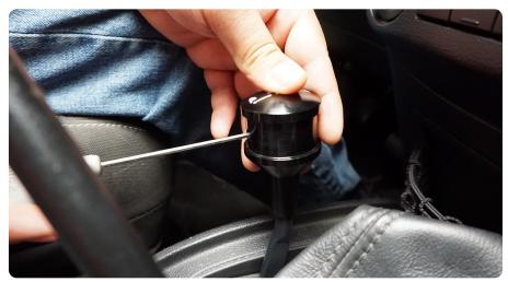
**STEP 5** | Replace the rubber grip to the DV8 shift knob.
