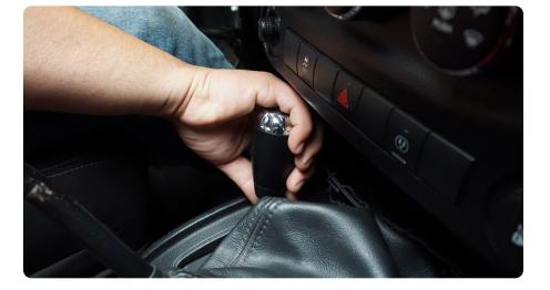
STEP 2 | Grab the knob and pull / twist upwards with force to remove the factory shift knob.
