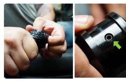
**STEP 3** Place your shift knob on shifter and with a 2.5 allen head, tighten the allen screw securing the shift knob.
