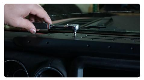
**STEP 7** Double check all hardware is secure and you are finished with your install of the DV8 JL/JT Dash Mount.
