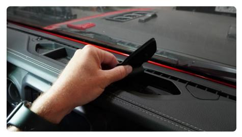
STEP 2 Using a phillips head screwdriver, remove the two factory OEM bolts.
