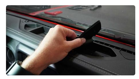
STEP 2 | Use a phillips head screwdriver, remove the two factory OEM screws.
