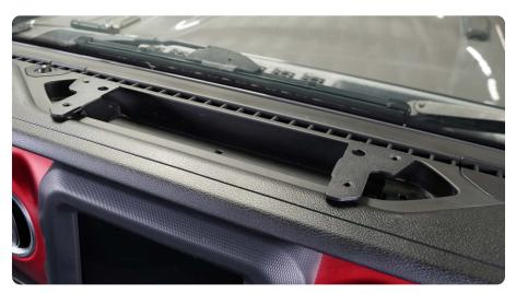
STEP 4 | Place the dash mount onto the installed brackets and ensure the beveled bolt holes align with the brackets.
