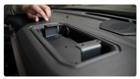
STEP 6 | With a firm grip, remove the factory dash pocket with the DV8 Dash Mount bracket in place.
