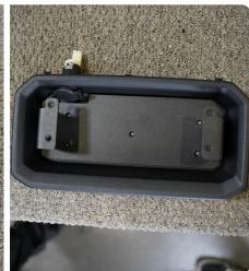
STEP 8 | Remove the DV8 mounting bracket.
