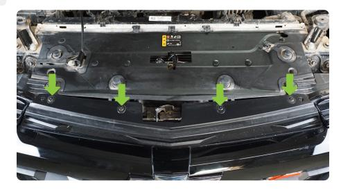
STEP  $2 \mid$  Use a T15 torx tool to remove the torx head bolts securing the inner fenders to the front bumper.
