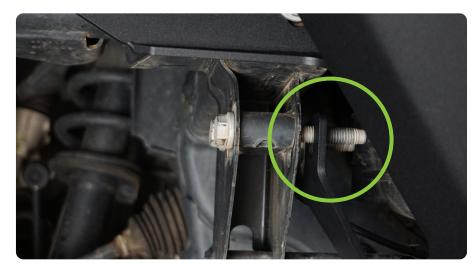
STEP 36 | Secure the winch plate supports in place using a #5 Allen tool.
