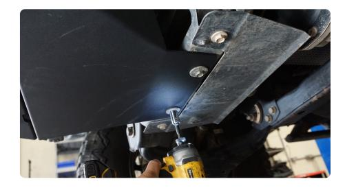
STEP 38 | With the bumper mounted, remove the factory bumper/ grille assembly lower fascia.
