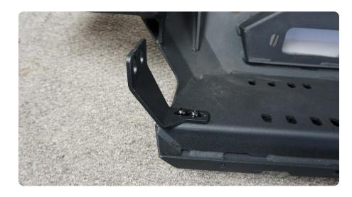
$\begin{array}{c|c} \text{STEP 16} & \text{Apply the provided peel} \\ \text{and stick foam pieces on to the bumper} \\ \text{wings as shown.} \end{array}$
