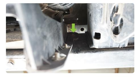
STEP 12 | Use your preferred cutting tool, to cut and remove the shutter shroud.
