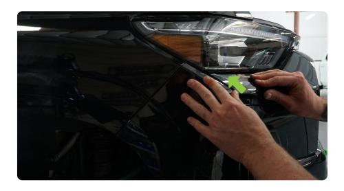
STEP 43 | Check that the cut is even across the bumper. Additional trimming my be required.
