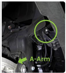
STEP 4 Disconnect the main bumper harness connector located behind the inner fender on the driver side of the vehicle. Pull the red locking clip back and rotate the gray lock to release, then pull.
