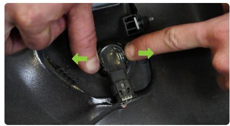
STEP 13 | Remove the sensor bezels from the bumper by pressing the small triangular tabs keeping the bezels in place, while gently pushing "out" towards the face of the bumper.
