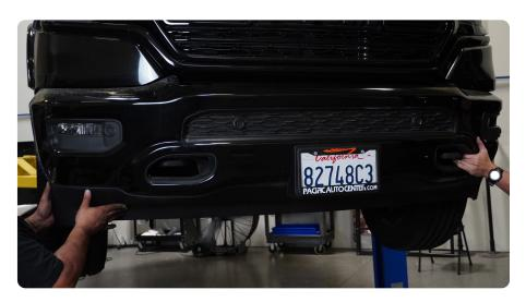
STEP 6 | Use an 18mm and 21mm socket to remove the (4) bolts securing the tow hooks and set them off the side.
