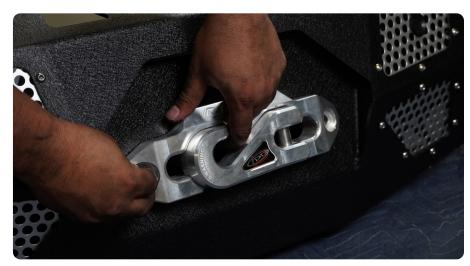
STEP 19 | Loosely install the new frame brackets using the provided M12x35 hardware and an 18mm socket and wrench.
