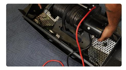
STEP 18 | If you are installing a fairlead, do so at this time using the hardware provided with the fairlead.
