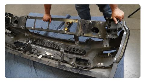
STEP 12 | Remove the sensors from their bezels by gently spreading the tabs that are securing it, and remove.
