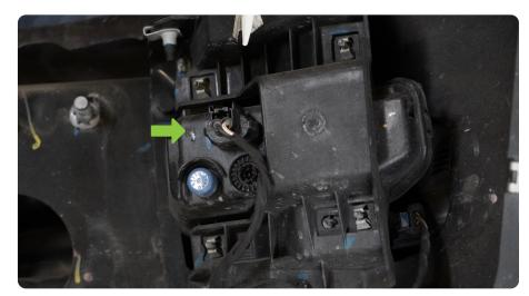
STEP 9 | Use a trim clip tool to remove the clips securing the wiring harness to the bumper brace.
