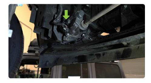
STEP 2 | Use an 8mm socket the remove the bolts securing the inner fender to the vehicle located in front of the tires on both sides of the vehicle.
