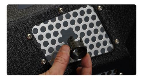
STEP 15 | Install the (2) center sensors into their bezels by gently pressing them, until they "clip" into place and are secure.
