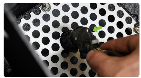
STEP 16 | Slide the outer sensors through the cutouts at the lower section of the bumper, to prepare for installation of the bumper on the vehicle.
