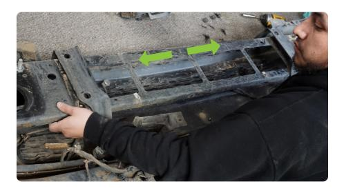
STEP 9 | Remove the sensor bezels by using a pry tool to press in the locking tabs at the side and pressing the bezel out.
