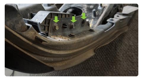
STEP 8 | Remove the parking sensors from the bumper bezels by gently prying the two tabs outward and pulling up on the sensor.
