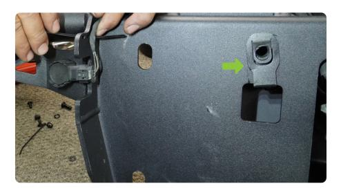
STEP 31 | With assistance, lift the bumper up to the truck ensuring all wiring is in place and not being pinched.
