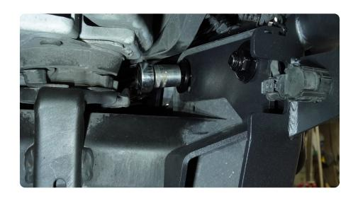
STEP 34 Using the M14 bolts provided, secure the bracket to the bottom of the frame. Using a 21mm, secure bracket to frame.
