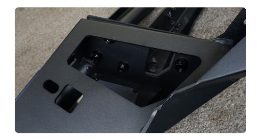
STEP 14 | Align the top of the wings to the center section of the bumper, using a 19mm and #8 allen head, tighten the wings into place.
