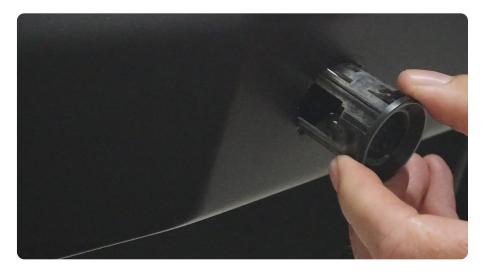
STEP 25 | Install the parking sensor back into the sensor bezel. Ensure tab on sensor aligns with notch in bezel.
