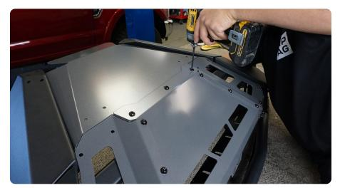
STEP 22 | Using the provided straps, secure the upper and lower skid plates together using the M8x20 hardware.
