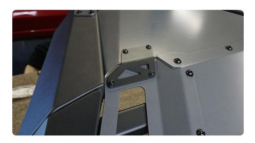
STEP 23 | If equipped with sensors, route the harness through the bumper placing each sensor in its relative position.
