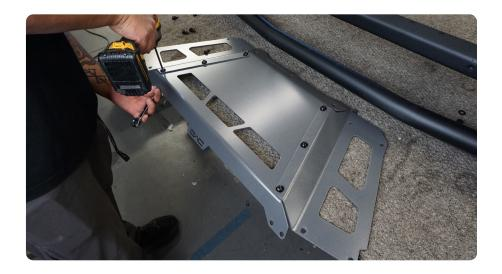
STEP 19 | Secure the upper portion skid plate to the bumper loosely using the same M8x20 bolts.
