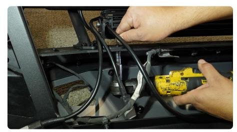
STEP 30 | Install the M12 nut clips onto the bumper as shown. These should "snap" into place.
