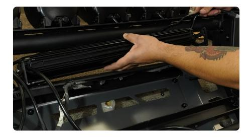
STEP 29 | The 20" light bracket will mount to the bumper utilizing the provided M6 hardware. Use a #4 and 10mm wrench to secure them into place.
