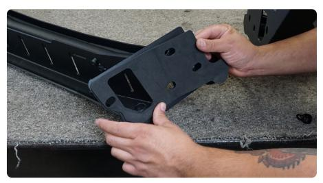
STEP 12 | Locate the two wings and loosely (hand tight) mount them to the center section of the bumper using the M12x30 allen head bolts. Use two flat washers and one nylock nut per bolt.
