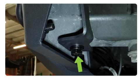
STEP 35 | Lift the bumper into place and adjust until the body lines are consistent and tighten all frame bolts with a #8 and 19mm socket.
