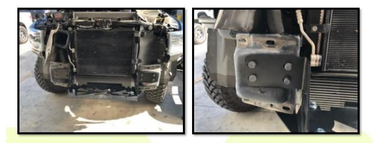
5. Locate and using provided hardware, install main bumper bracket on each side. These are held on by (3) three bolts on each side and go over the winch plate bracket. Using the studs on these brackets, you will then install the bumper center section bracket. Ensure that these are installed like the below images. (NOTE: If you are planning on installing a winch, now is the time to do so)
