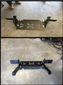
4. Install winch plate assembly onto truck using factory hardware to mount main winch plate bracket to factory bumper plates. Center winch plate assembly onto truck and tighten down. Leave lower support brackets unbolted for now.
