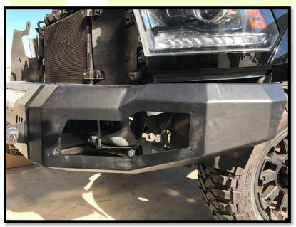
8. Once both wings are attached and fastened securely, locate the wing support brackets. Using provided hardware, attach to this to the inside of each bumper wing loosely and do not attach the opposite side to the truck at this moment.
