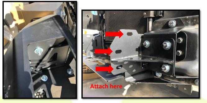
7. Once center section is loosely attached, attach both wings onto center section using supplied hardware. <u>Ensure to align them with center section</u> and tighten them down. <u>Do not</u> attempt to line up the entire bumper with body line of truck at this point.
