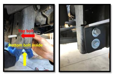
11. Loosely attach skid plate to bumper using supplied hardware. Using the 4" long bolts provided, attach skid plate to backside of frame horn that the winch plate support bracket bolted to. The bolt will be at an angle. You can tighten down at an angle without any damage or integrity loss, or you can open up the hole to level out the bolt. Secure all skid plate bolts.
