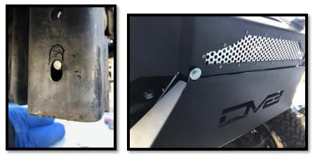
12. Remove front bolt and install wing support bracket reusing factory bolt. Once secured, tighten down <u>ALL hardware</u> for bumper. Reinstall factory grill.
