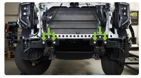
STEP 18 | Use an 18mm socket and an adjustable wrench to remove to remove the front recovery hooks.
