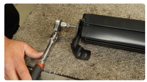
STEP 50 | Mount the light bar within the bumpers center section using a #4 allen tool and 10mm wrench with the provided M6 hardware.
