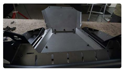
STEP 31 | Loosely mount the lower skid plate frame to the bumper wings/lower skid plate using a #5 allen tool, 13mm wrench and the provided M8x20mm hardware.
