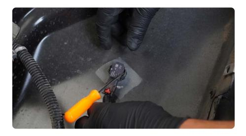
STEP 24 | With the harness and sensors removed, push in the two retainer tabs on the bezels and push them out the front of the bumper.
