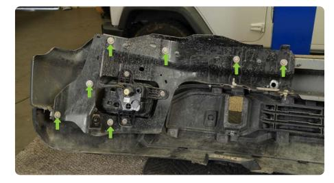
STEP 23 | Using a trim tool, remove the clips holding the harness to the bumper.
