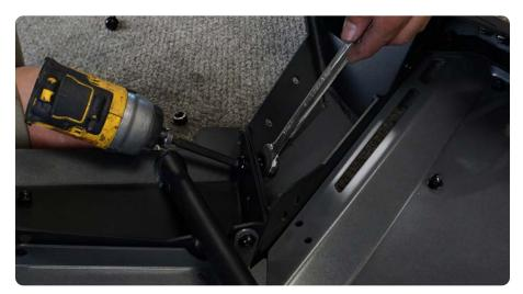
STEP 32 | Loosely mount the front cross-member mounting bracket to the bumper using a #5 allen tool and the provided M8x20 hardware.
