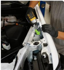
STEP 8 | Carefully start to pull the lower fascia away from the vehicle with a firm grip.
