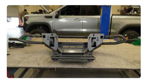
$\begin{array}{c|c} \text{STEP 36} & \text{I} & \text{Install the provided M12} \\ \text{clip nuts onto the bumper} \end{array}$
