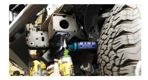
STEP 58 Using a 18mm socket and 19mm wrench, secure the recovery point to the lower bumper support/ frame rail crash-bar.
