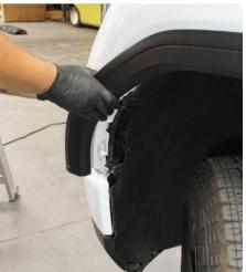
STEP 6 Using a 8mm socket, remove the bolt that secure the lower fascia to the fender on each side.
