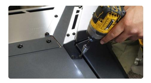
STEP 34 | Loosely mount the center support bar as shown using a #5 allen tool and 13mm wrench with the provided M8x20 hardware.
