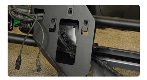
STEP 43 | The passenger side inner parking sensor wiring harness will need to be lengthened.
