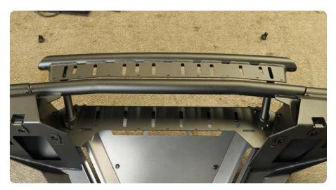
STEP 39 | If equipped, route the driver side parking sensor through the bumper and over to the driver side sensor bezel hole in the bumper.
