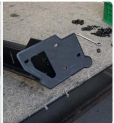
STEP 26 | Loosely mount the wing to the bumpers center section using a #5 allen tool and 13mm wrench using the M8x20 hardware provided.
