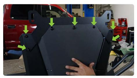
STEP 33 | Loosely mount the skid plate support brackets using a #4 allen tool and 10mm wrench, with the provided M6x20 hardware.
