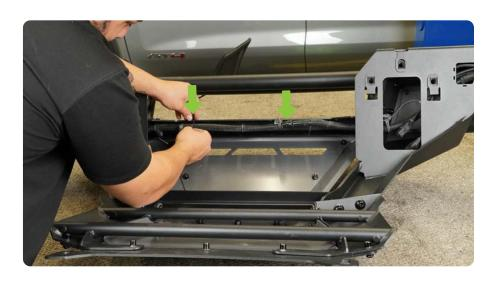
STEP 49 If you are planning to run a light bar in the center of the bumper, mount the provided light bar brackets to your light bar using the hardware provided with the light.
