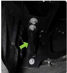
STEP 14 | Use an 18mm socket to remove the (2) lower bumper mounting bolts on the inside of the frame rails.
