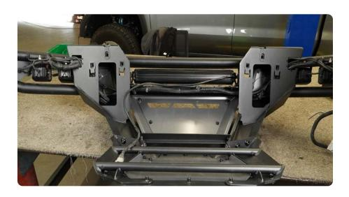
STEP 51 | If you wish to run light along the push bar, install your lights at this time using the hardware included with the lights.
