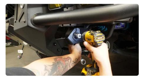
STEP 59 | Using the factory skid plate to cross-member bolts, secure the DV8 skid plate to the cross member.
