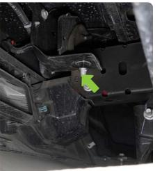
STEP 15 Use a 10mm socket to remove the (4) bolts securing the bumpers lower valance.
