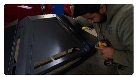
STEP 30 | Loosely mount the lower skid plate using a #5 allen tool and the provided M8x20mm hardware.
