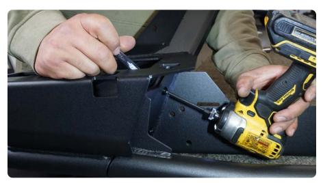
$\begin{array}{c|c} \text{STEP 27} & \text{With the wings mounted} \\ \text{flip the bumper as shown.} \end{array}$
