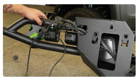
STEP 40 | Install the sensor bezel previously removed, into the cutout on the DV8 bumper.
