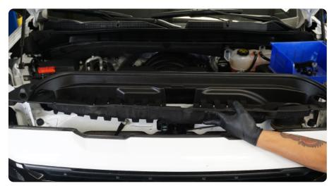
STEP 3 Using a 10mm socket, remove the (4) bolts securing the top of the grille to the vehicle.
