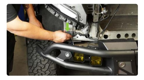
STEP 61 | Ensure all light wiring is tucked away from the top of the bumper.
