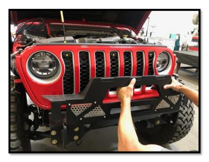
4. Align the 8 holes on the top of the bumper with the winch plate below. Secure the 4 holes closest to the center with our taper allen head bolts and rock washers provided in the hardware kit.
