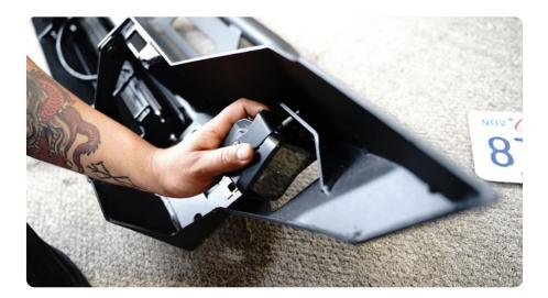
If you are installing a winch, do so at this time using the hardware provided with the winch.
