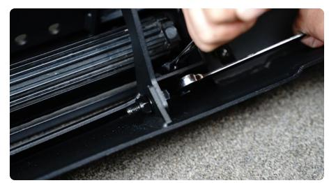
STEP 10 | Install the flat nuts onto the bumper by pressing them into place.
