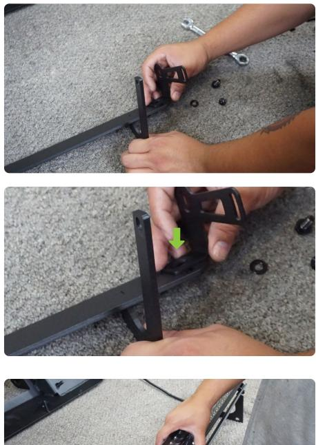
**STEP 9** | Install the light bar to the mounting bracket using the hardware that was provided with the light.
