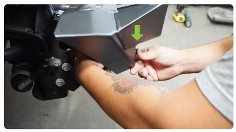
STEP 12 | Ensure main bumper bolts are torqued to 27ft lbs. Double check fitment and all hardware is secure.
