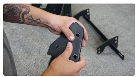
STEP 8 | Install the wings using the provided M10x30 Hex Hardware with a 16mm socket and 17mm wrench.
