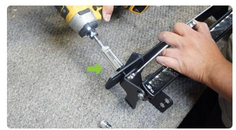
STEP 11 | Perform a test fit of the cross bar without installing any hardware to determine if the light bar needs to be adjusted.
