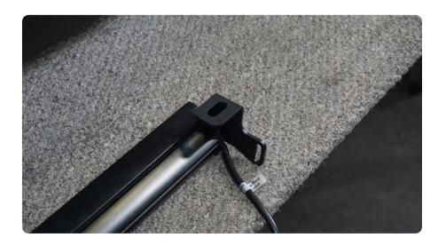
STEP 12 | Install the light bar mounts to the cross brace using the provided M10 hardware with a 16mm socket and 17mm wrench.
