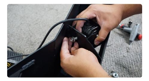
STEP 14 | With assistance, lift the bumper to the vehicle while aligning the studs to the mounting holes.
