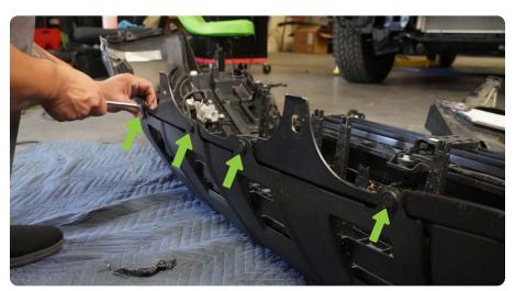
**STEP 13** With all trim clips freed, use a Philips head screw driver to remove the (2) Philips head screws that secure the center lower valance to the grille assembly.
