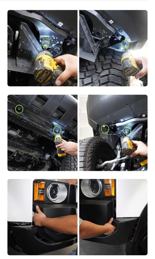
**STEP 7** With a firm grip, pull the bumper/grille assembly away from the vehicle to release any push clips that secure the bumper/grille assembly.
