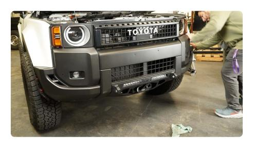
**STEP 23** Check the fitment of the bumper/grille assembly around the DV8 Centric Front Bumper.
