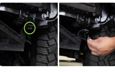
**STEP 10** Use a trim clip tool to remove the push pin that secure the plastic air guards to the crash bar.
