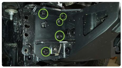
**STEP 22** | Install the factory bumper/ grille assembly back on to the vehicle and test fit the grille assembly with the DV8 bumper in place.
