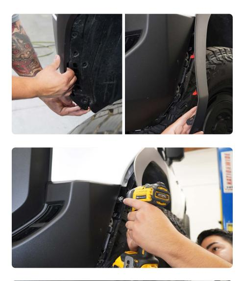
**STEP 5** Use a trim clip tool to remove the (2) push pins behind the fender flare on each side.
