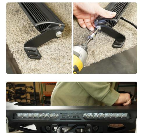
STEP 19 | Install the light bar assembly onto the bumper as shown, loosely secure the light bar brackets to the bumper using the provided M6 Hardware.
