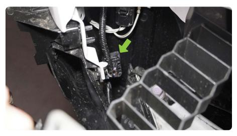
STEP 26 | If you are planning to run the factory skid plate you will need to cut off the (3) mounting tabs as shown using your preferred cutting tool.
