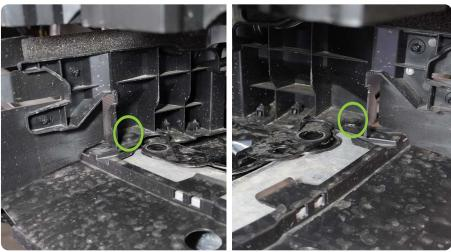
STEP 11 | Use a 17mm socket to remove the (10) hex bolts that secure the crash-bar to the vehicle.
