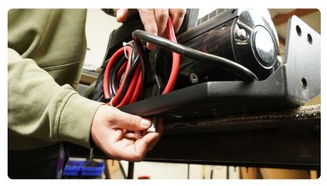
STEP 17 | Install your chosen fairlead onto the DV8 front bumper before mounting the winch and winch plate.
