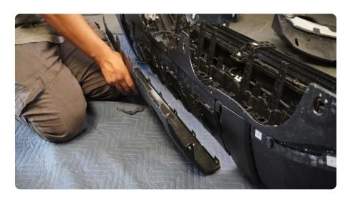
Use your preferred cutting tool to cut out the bumpers center fascia section following the center lower valance grooves.
