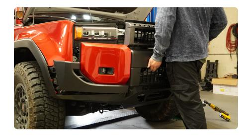
STEP 28 | To obtain the ultimate fit and finish, trim the grilles lower bumper valance to match the bumper wing. We recommend leaving a 1/8 inch gap between the lower bumper valance and the DV8 bumper to account for body flex.
