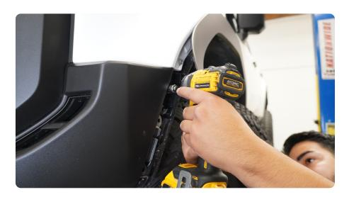
STEP 5 | Use a trim clip tool to remove the (2) push pins behind the fender flare on each side.
