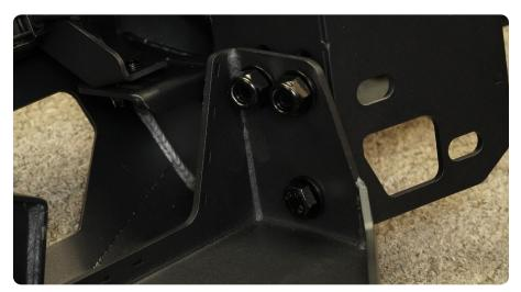
STEP 22  $\mid$  Mount the winch to the DV8 winch plate using the hardware provided with the winch.
