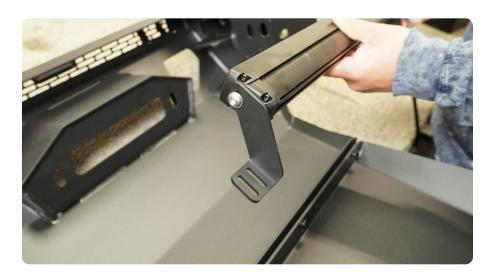
STEP 20 | Center the light bar into the bumper as shown. Using a #4 allen too, 10mm socket/wrench and the provided M6 hardware, secure the light bar brackets in place.
