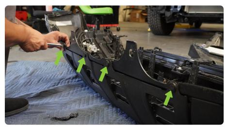
STEP 13 | With all trim clips freed, use a Philips head screw driver to remove the (2) Philips head screws that secure the center lower valance to the grille assembly.
