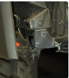
STEP 25 | With assistance, lift and mount the bumper onto the vehicle, loosely using the provided M10 and M14 Hex bolts.
