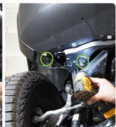
STEP 7 | With a firm grip, pull the bumper/grille assembly away from the vehicle to release any push clips that secure the bumper/grille assembly.
