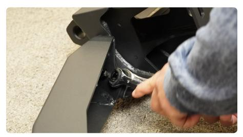
STEP 18 | Using the provided M8 allen head bolts and a #5 allen tool, loosely secure the skid plate to the bumpers center section.
