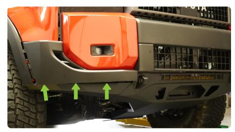
STEP 29 | Once you have finished trimming the lower bumper valance, ensure all grille assembly clips have been pushed back into place.
