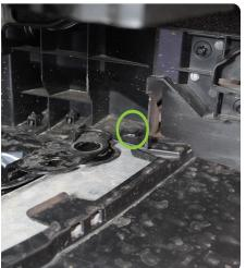
STEP 11 | Use a 17mm socket to remove the (10) hex bolts that secure the crash-bar to the vehicle.
