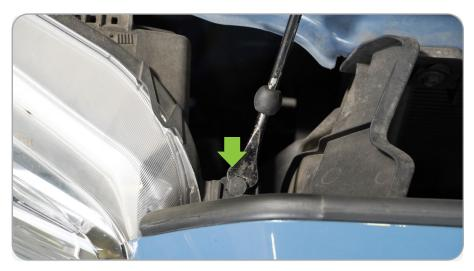
STEP 3 | Use the push pin removal tool to unplug the air sensor harness on the backside of the grille.
