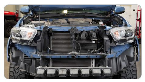
STEP 11 | Disconnect the wheel well orange clips crash bar support
