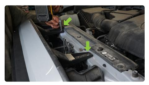
$\begin{array}{c|c} \text{STEP 34} & \text{Re-install the factory push} \\ \text{clips securing the grille to the vehicle.} \end{array}$
