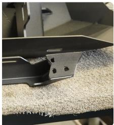
STEP 26 | If planning to run a light in the bull bar, install the light using the brackets included in the bumper kit and the hardware provided with the light.
