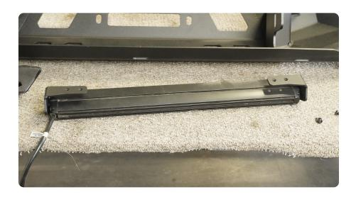
STEP 27 | Center the light onto the bull bar. Using a #4 Allen tool and the provide (4) M6 Allen head bolts secure the light to the bull bar.
