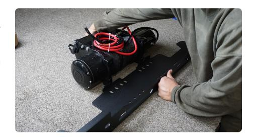
STEP 30 | Lift the winch plate/winch up to the vehicle and loosely secure using the factory hardware.
