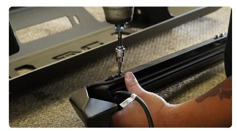
STEP 28 | Install the bull bar using a 10mm wrench, #4 Allen head tool, (6) M6 Allen head bolts and (6) Nylon lock nuts.
