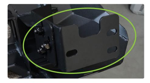
STEP 25 | If you are planning to run the optional bull bar, install the provided foam pieces on to the bull bar mounting base as shown.
