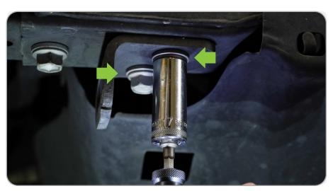
STEP 16 | Using the 17mm socket, remove the remaining bolt on the underside of the front frame crossmember to remove the frame extension. Repeat on opposite side.
