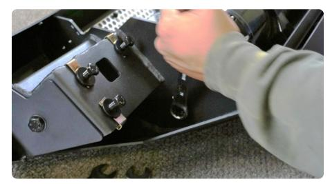
STEP 18 | If you are running pod lights, install them at this time using the hardware provided with the lights.
