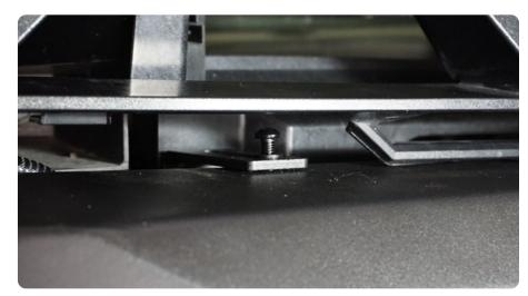
STEP 55 | Re-install factory clips located next to the wiring plugs at both ends of the vehicle behind the headlight.
