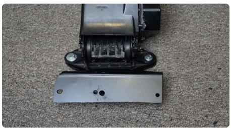
STEP 49 | Install the air dam bracket onto the horizontal cross brace using the provided M6 hardware and a 4mm allen bit. Connect the air dam motor wiring plug.
