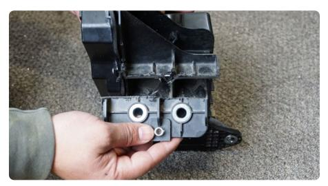
STEP 42 | Trim the small remaining mounting tab off the motor as shown.
