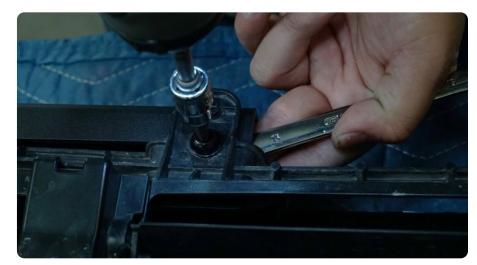
STEP 35 | Use a 10mm socket and the factory bolts to install the shutters.
