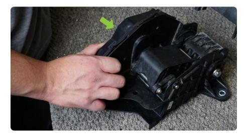
STEP 44 | Use a 10mm socket to remove the bolt securing the cooling hoses to bracket located in front of the radiator on the passenger side.
