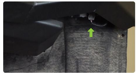
STEP 58 | Connect the wiring located on the passenger side of the vehicle underneath the upper mounting bracket on the grille. (From Step 8)
