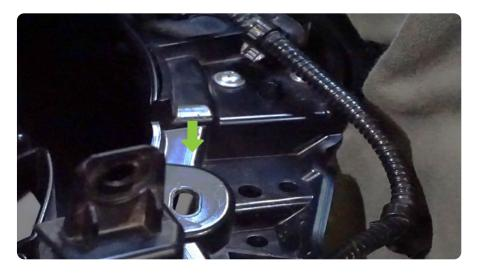
STEP 57 | Connect the wiring located behind the bumper in the fender well on both passenger and driver side of vehicle. (From Step 7)
