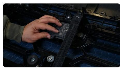
STEP 28 | Remove upper mounting bracket from the grille by pulling it away from the grille to release the clips.
