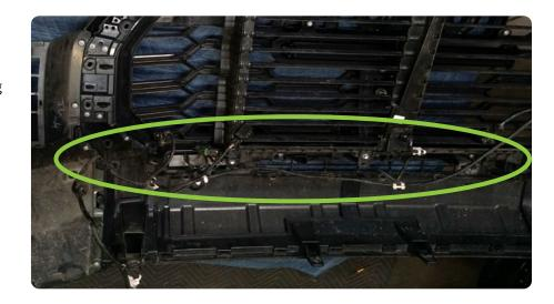
STEP 25 | Install the sensor plugs into the bumper correlating to the factory locations.
