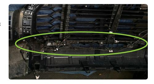
$\begin{array}{c|c} \text{STEP 25} & \text{Install the sensor plugs} \\ \text{into the bumper.} \end{array}$
