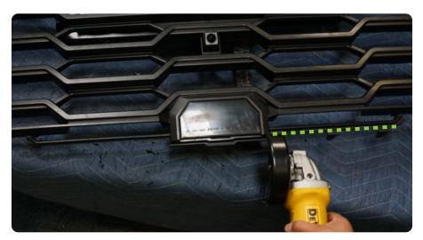
STEP 30 | Use an angle grinder to grind a small section off the bottom corners of the grille.
