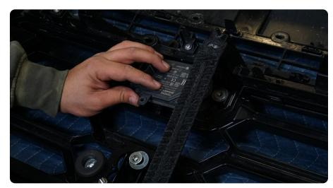
STEP 28 | Remove upper mounting bracket from the grille by pulling it away from the grille to release the clips.
