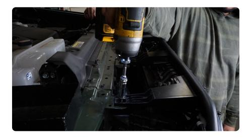
STEP 54 | Use the provided M6 hardware and a 4mm allen bit to secure the lower section of the grille to the bumper. The same tabs from step 36.
