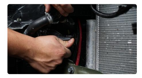
hardware with a 4mm allen bit and 10mm wrench to secure the air dam motor to the provided bracket.
