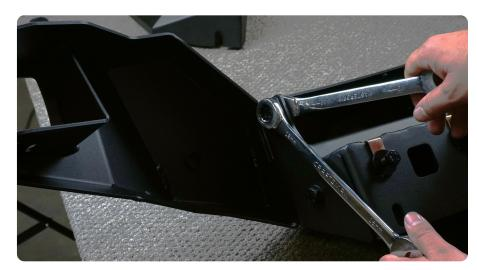
STEP  $16 \mid$  Install the M10 flat nuts on the bumper by pressing them into place.
