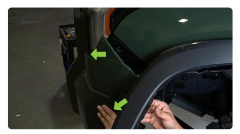
STEP 4 | Reach behind and underneath the bumper to remove the black plastic trim by pressing out the clips from the inside.
