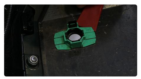
STEP 23 | Clean the residue off the sensor plug using a blade so that when installed, it will sit flush.
