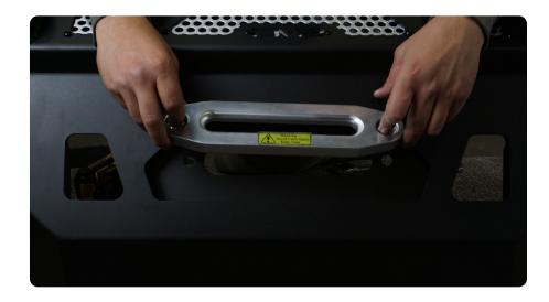
STEP 17 | Install the winch plate using the provided M14 hardware and a 21mm and 19mm wrench.
