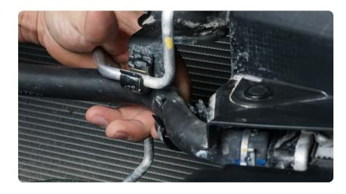
STEP 46 Use a 10mm socket to remove the bolt securing the vertical cross brace. Slip the cooling hose behind the cross brace and re-secure using the factory hardware.
