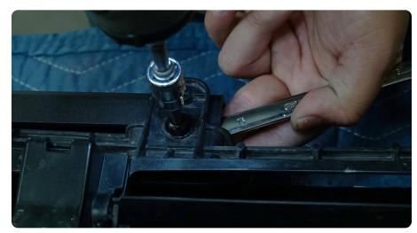
$\begin{array}{c|c} \text{STEP 35} & \text{Use a 10mm socket and} \\ \text{the factory bolts to install the shutters.} \end{array}$
