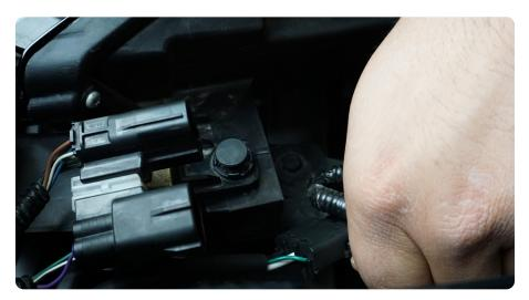
STEP 6 | Disconnect the wiring plug located between the bumper and radiator in the center section of the vehicle.
