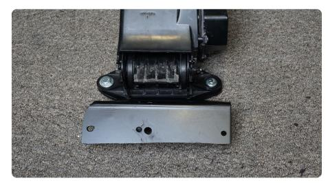
STEP 49  $\mid$  Install the air dam bracket onto the horizontal cross brace using the provided M6 hardware and a 4mm allen bit. Connect the air dam motor wiring plug.
