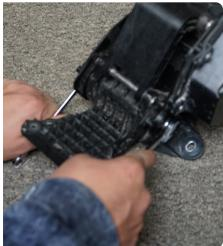
STEP 38 | Remove the black caps, the white plastic spacers and the spring from the inside, and set the arm off to the side.
