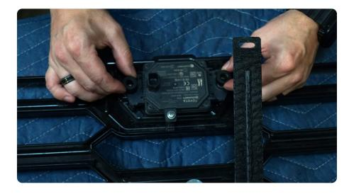
STEP 34 | Secure the shutters to the provided bracket using the provided M8 hardware with a 5mm allen bit and 13mm wrench.
