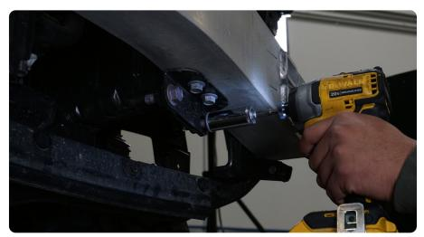
STEP 12 | Use a 10mm socket to remove bolts securing the vertical cross braces from the vehicle.
