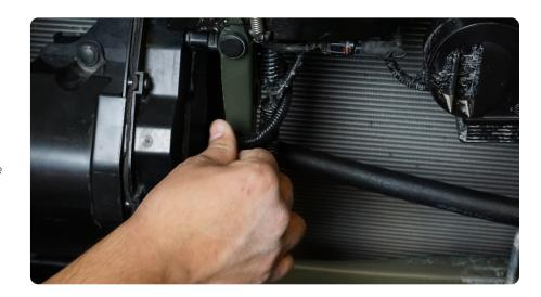
STEP 51 | Place the wiring harness into the bumper and run the wires so that the sensors are at their approximate location of install. Secure the wiring in a safe location.
