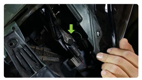
STEP 8 Disconnect the wiring plugs located behind the grille on the passenger side of the vehicle underneath the grille's upper mounts.
