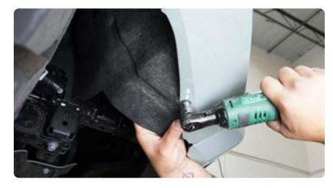
STEP 43 Attache the Bumper support brackets using a 5mm Allen bit, a 13mm wrench and the provided M8 hardware.
