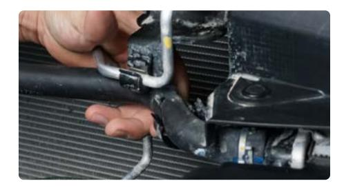
STEP 31 | Use a 10mm socket to remove the bolt securing the vertical cross brace. Slip the cooling hose behind the cross brace and re-secure using the factory hardware.
