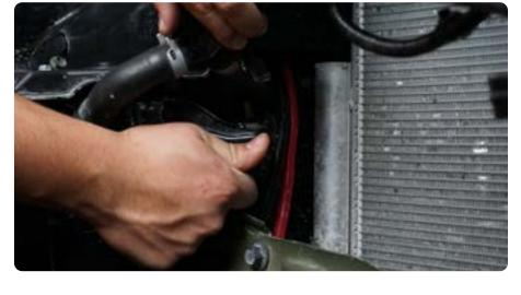
STEP 33 | Use the provided M6 hardware with a 4mm allen bit and 10mm wrench to secure the air dam motor to the provided bracket.
