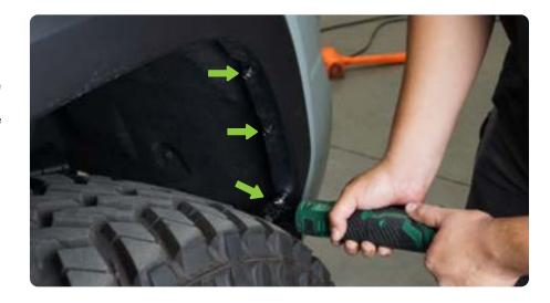
STEP 42 | Reattach the bumper to the fender liner using a 10mm socket and factory hardware previously removed.
