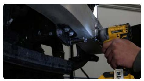
STEP 11 | Use a 10mm socket to remove bolts securing the vertical cross braces from the vehicle.
