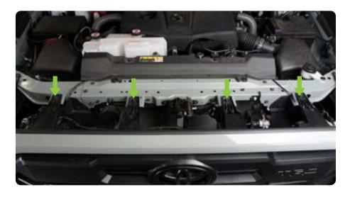
STEP 45 | Install all push pins and reconnect all wiring harness's previously removed or disconnected.
