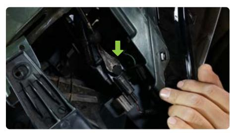
STEP 7 Disconnect the wiring plugs located behind the grille on the passenger side of the vehicle underneath the grille's upper mounts.
