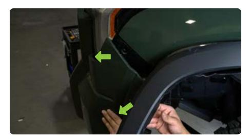
STEP 3 | Reach behind and underneath the bumper to remove the black plastic trim by pressing out the clips from the inside.
