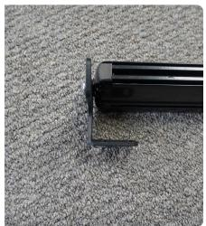
STEP 11 | Install the light bar with the brackets on the bumper using the provided M6 hardware.
