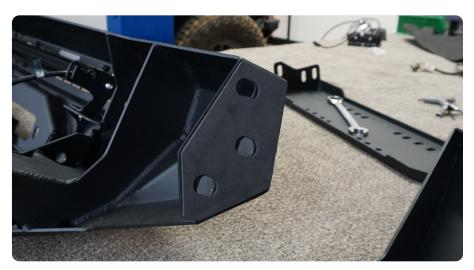
STEP 9 | Install the bumper wings using the provided M14 hardware.
