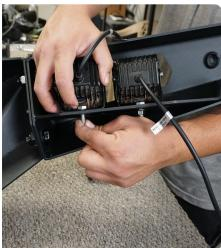
STEP 16 | Install the parking sensors into your new bumper in the same position/orientation as they came off the OEM bumper.
