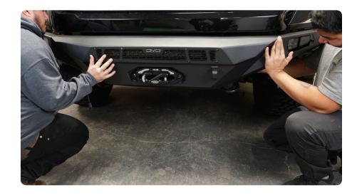
STEP 18 | Secure the bumper using factory hardware and a 14mm socket.
