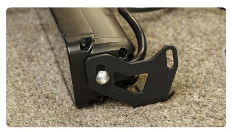
STEP 21 | Using a #4 allen tool and 10mm wrench, mount the light bar brackets to the bumpers center section using the provide M6 hardware.
