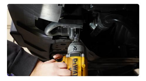
STEP 5 Use a 14mm wrench or deep socket to remove the 4 bumper mounting nuts on each side.
