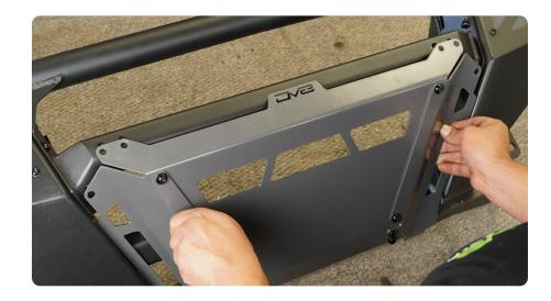
STEP 15 | Loosely secure the skid plate section to the tube assembly using the provided M8 hardware and a #5 allen tool.
