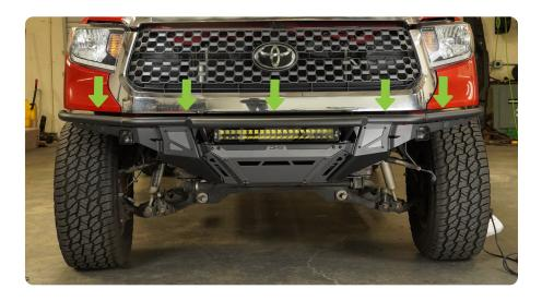
STEP 26 | Loosen the bolts that secure the bumper to frame rail brackets using a 17mm socket.
