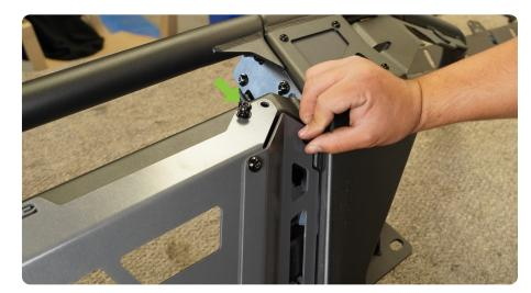
STEP 16 | At the bottom of the skid plate, use the provided M6 hardware and a #4 allen tool to secure the skid plate to the lower cross bar.
