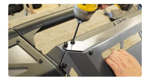
STEP 18 | The DV8 tube bumper comes with an optional push/light bar. If you wish to run the push/light bar mount the push/light bar using the provided M8 hardware and a #6 allen tool.
