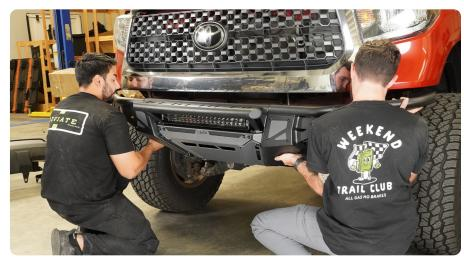
STEP 24 | Secure the DV8 tube bumper to the frame rails using the factory hardware and a 14mm socket.
