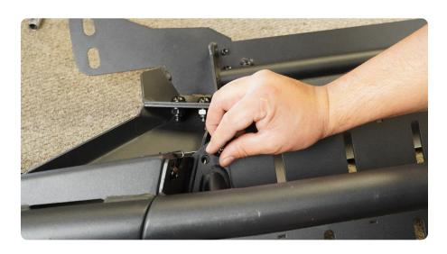
STEP 19 | Attache the bumper mounting bracket to the wings using the provided M10 hex head bolts.
