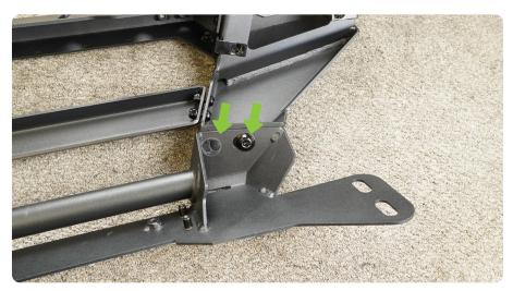
STEP 11 | Before securing any hardware, ensure the upper tube are aligned and level.
