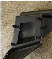
STEP 9 Using a #5 allen tool and 13mm socket with the provided M8 attach the wings to the bumpers center section that houses the light bar.
