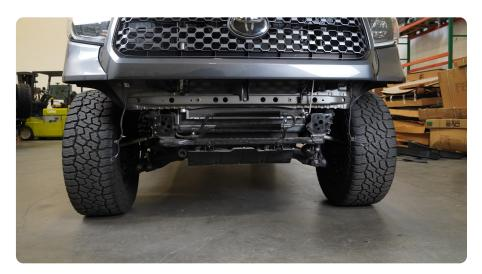
STEP 7 Remove the parking sensors from the OEM Bumper. First, unplug the sensor then, slide the white plastic piece to the side. Push the sensor out the front of the bumper.
