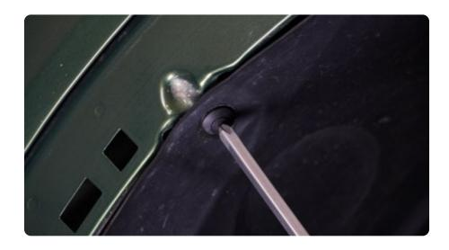
STEP 9 After installing the seal onto the rear fender in the same fashion, mount onto vehicle using #4 allen, 10mm wrench/socket with M6 hardware.
