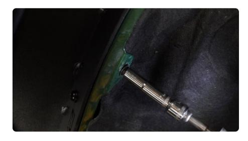
STEP 7 | The rear will be similar to the fronts by removing the factory fender. These are easily removed by twisting the small latches until latch becomes loose. Once all are loose, pull fender away from Bronco until hidden clips release.
