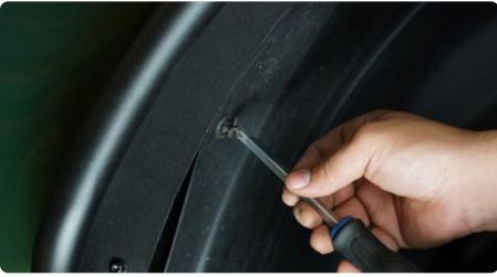
STEP 12 | After all fenders are installed, using a sharp razor, trim any excess seal to preference making sure to cut towards the fender, not the body to avoid damage to the vehicle.
