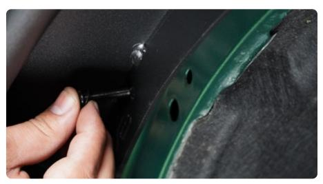
**STEP 5** Once all fender hardware is installed, align the fender of the vehicle and secure hardware.
