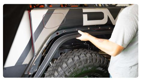
STEP 13 | Install the fender flare onto the vehicle using the provided M6x25 hardware with a 4mm allen bit (and 10mm wrench if using nuts).
