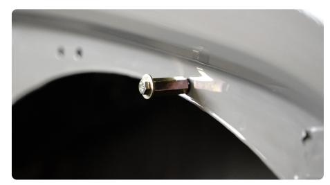
STEP 18 Use a 12mm wrench to hold the spacer while tightening with a 10mm socket. Tighten slowly until the nutsert is set properly. Do not over tighten.
