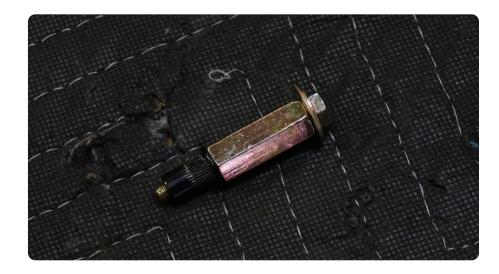
STEP 17 | Slide the nutsert tool with the nutsert into the mounting hole. Ensure the flange of the nutsert is flat against the vehicle prior to tightening.
