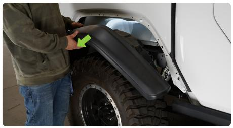
**STEP 7** Use a trim clip tool to remove the clips along the edge of the fender that remained in the vehicle.
