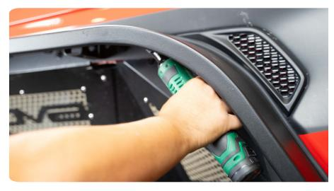
STEP 12 | Route and secure the wiring to your preference and install the new turn signal into the factory connector.
