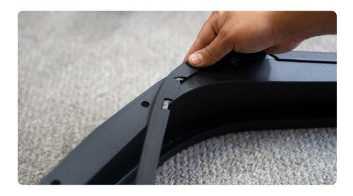
STEP 11 | Install the fender flare onto the vehicle using the provided M6x20 hardware with a 4mm allen bit.
