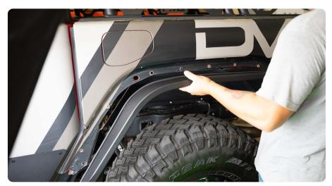
STEP 14 | Install the fender flare onto the vehicle using the provided M6x25 hardware with a 4mm allen bit (and 10mm wrench if using nuts).
