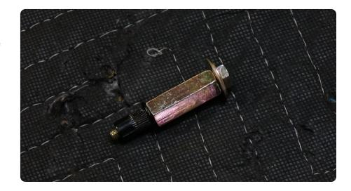
STEP 18 | Slide the nutsert tool with the nutsert into the mounting hole. Ensure the flange of the nutsert is flat against the vehicle prior to tightening.
