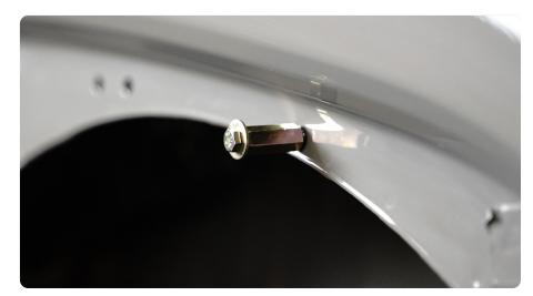
STEP 19 Use a 12mm wrench to hold the spacer while tightening with a 10mm socket. Tighten slowly until the nutsert is set properly. Do not over tighten.
