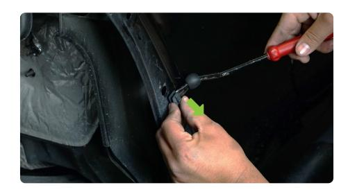
STEP 6 Use a trim clip tool to remove the five trim clips located along the interior of each rear inner fender.
