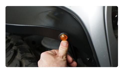
**STEP 17** | Connect the light to the factory connector and secure it out of the way using a zip ties.
