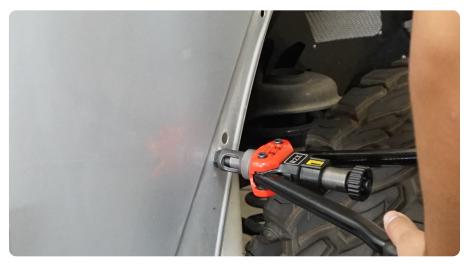
STEP 19 | Loosely secure the fenders to the vehicle using the provided M6 hardware. Check that the gasket does not move out of place during install.
