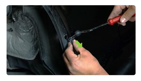
**STEP 6** Use a trim clip tool to remove the five trim clips located along the interior of each rear inner fender.
