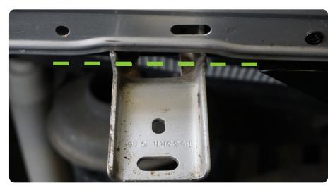
**STEP 13** | Loosely install the front fenders using the provided M6 hex head hardware. Check that the gasket does not move out of place during install.
