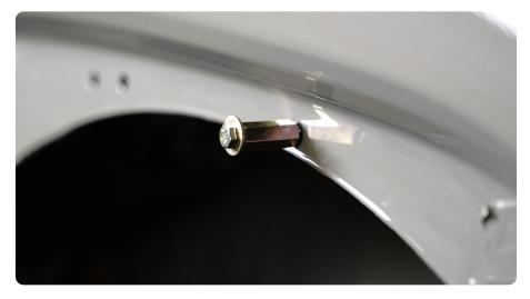
STEP 23 Use a 12mm wrench to hold the spacer while tightening with a 10mm socket. Tighten slowly until the nutsert is set properly. **Do not over tighten.**
