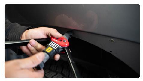
**STEP 19** | Loosely secure the fenders to the vehicle using the provided M6 allen head hardware. Check that the gasket does not move out of place during install.
