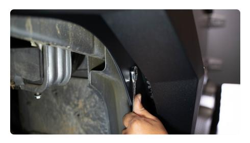
STEP 15 | Pull the rubber grommet off the light and slide the light through to mounting hole on the fender. Then pull the grommet through the hole until it is evenly seated in the hole.
