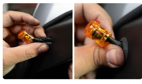
**STEP 16** | Connect the light to the factory connector and secure it out of the way using a zip ties.
