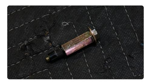
STEP 22 | Slide the nutsert tool with the nutsert into the mounting hole. Ensure the flange of the nutsert is flat against the vehicle prior to tightening.
