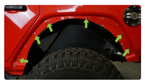
STEP 15 | Install the Rear Fender Delete onto the vehicle using the provided M6x25 hardware with a 4mm Allen tool (and 10mm wrench if using nuts).
