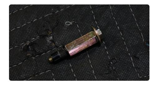
STEP 19 | Slide the nutsert tool with the nutsert into the mounting hole. Ensure the flange of the nutsert is flat against the vehicle prior to tightening.
