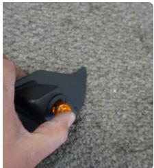
STEP 11 | Route and secure the wiring to your preference and install the new turn signal into the factory connector.
