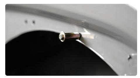
STEP 20 Use a 12mm wrench to hold the spacer while tightening with a 10mm socket. Tighten slowly until the nutsert is set properly. Do not over tighten.
