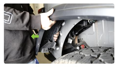
STEP 7 Use a trim clip tool to remove the clips along the edge of the fender that remained in the vehicle.
