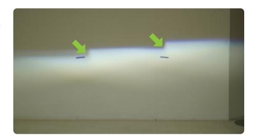
STEP 18 | Using a medium size phillips screw driver, rotate the adjuster to move the light up and down.
