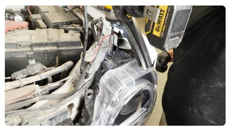
STEP 7 | With the bolts removed, pull the light out of the Bronco and unplug the light from the harness.
