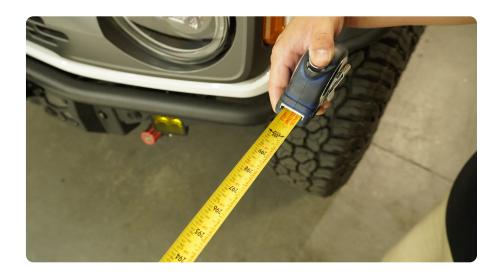
STEP 16 | Measure the centerline of your headlight. If 36" or lower, mark the same height on the wall.
