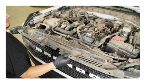
STEP 2 | Use a 10mm socket, remove the bolts along the top side of the grille.
