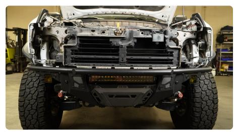
STEP 9 | Since the side market light is removed with the factory headlight, the DV8 kit comes with a new marker light. They are marked "L" and "R". Using the provided phillips head screws, mount the marker lights to the grille as shown.
