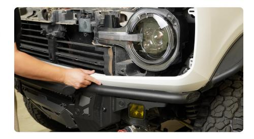
STEP 13 | Next will be to install the grille. Prior to placing the grille on the vehicle, plug the side marker lights into the headlights.
