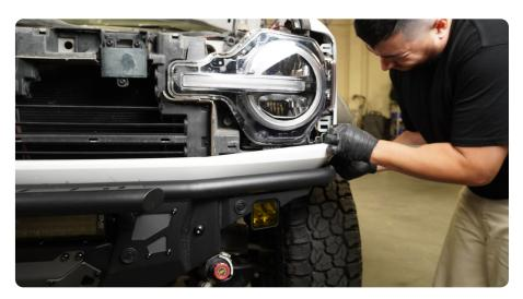
STEP 6 Using 8 and 10mm sockets, unbolt the headlight.
