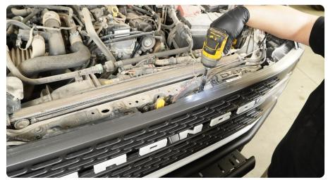
$\begin{array}{c|c} \text{STEP 3} & \text{Unclip the plugs for camera} \\ \text{and washer if equipped.} \end{array}$
