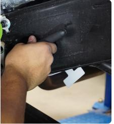
STEP 12 | Install the rear portion of the inner fender and align it with the holes at the bottom.
