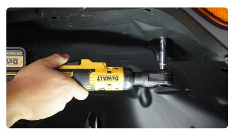
STEP 3 | Remove the plastic liner by holding the fender near the lip and pulling down and out.
