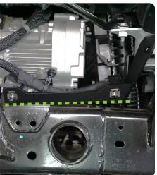
STEP 8 | Tuck the wiring for the fender light by pushing the plug up into wheel well.
