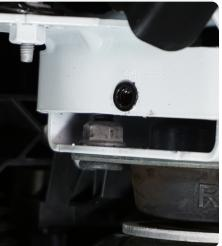
STEP 7 | Place the mounting bracket over the nutsert and secure the bracket in place with the provided M6 hardware and a #4 Allen tool.
