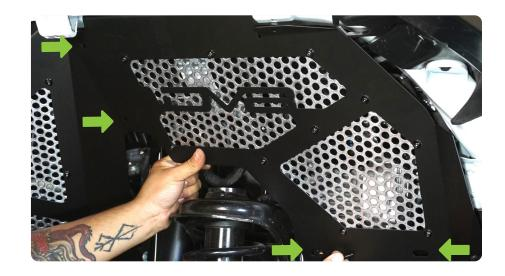
STEP 15 | Use the provided serrated nut to and M6 hardware to secure the top portion of the fender.
