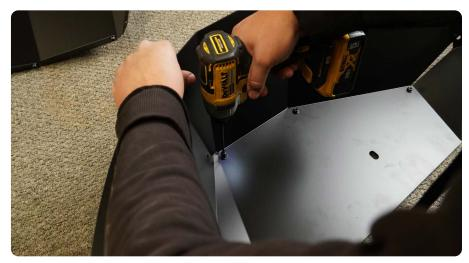
**STEP 5** Secure the side of upper panel to the lower panel using the provided M6x20mm Allen head bolts, M6 Nylon lock nuts, #4 Allen tool and a 10mm wrench.
