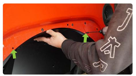
Secure the inner fender to the fender panel using the provided M5x30mm Allen head bolts and the pre-installed M5 nutserts.
