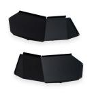
**STEP 1** Use a trim clip tool to separate the inner fender from the fender.
