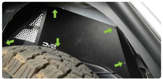
STEP 5 Using a 1/8 inch drill bit, drill a pilot hole for each of mounting screws.
