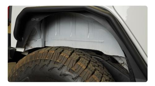
STEP 2 | Place the DV8 inner fender behind the wheel as shown.
