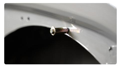
STEP 11 | Use a 12mm wrench to hold the spacer while tightening with a 10mm socket. Tighten slowly until the nutsert is set properly. Do not over tighten.
