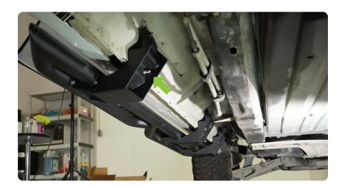
STEP 2 | Use the provided M8 hardware to loosely secure the DV8 OE Plus Step to the vehicle.
