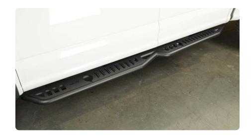
STEP 4 | Repeat steps 1-3 for the passenger side and double check that all hardware is secured.
